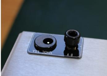
IV) Use 14mm spanner to remove nut on DC socket, then remove cable
