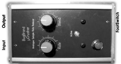
The **BugBrand**  $\mu$ Crusher is a compact Analogue Sample Rate Reduction audio processing device and achieves this effect by use of a Sample & Hold circuit clocked at audio rates.
