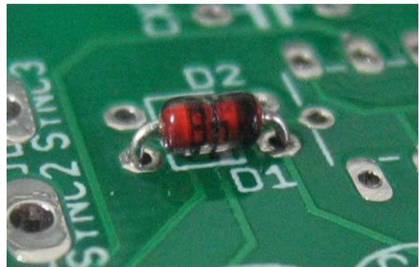
Turn the board over making sure the diode stays in position – you can splay the legs out slightly to prevent the component moving about. Now have a go at soldering, remembering the order: clean tip -> tin tip -> heat join -> flow solder -> clean, tin and replace. If all goes correctly you should have two nice clean solder joints. If you've done that ok then you can snip the leads off just above the join – nice and neat.
