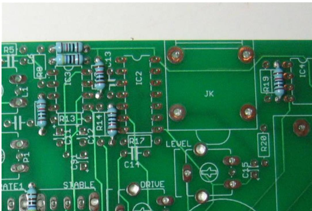
And finally the single 12k (R13) and the nine 100ks - R4, R5, R6, R7, R8, R14, R17, R19, R20:
