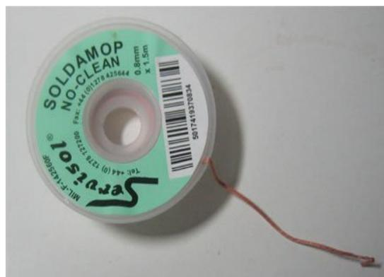
Desoldering braid draws up molten solder by capillary action. You put the braid on top of the solder to be removed and press the iron tip on top, melting the solder into the braid. It is generally necessary to pull the braid across the join to remove all the solder – a technique that takes a little practice!
