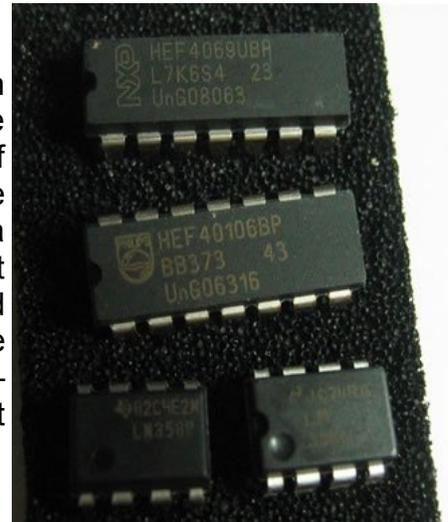
*Technique 1* – pick up the chip and orientate it. Gently position the legs of one side into one side of the IC holder. Holding the chip at an angle of about 35deg, apply a gentle pressure in the direction shown so that the legs bend very slightly – don't push too hard or the legs will all bend out of shape! Gradually bring the other side of the IC down to locate the rest of the legs into their sockets – once things are in position, apply a final downward pressure to fully seat the chip.
