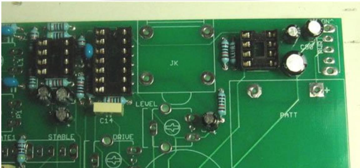
Time for the controls – the pots. You can leave off the spindle dials until the end, so put them back in the bag and sort out the different value pots. There should be one with 10k marked, one with 1M marked and then eight remaining all with 100k.
