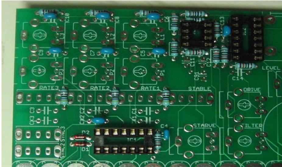
On to the poly box caps (again, not polarized). These have a slightly confusing number system (this actually varies a lot between different types and makes of capacitor) so go slowly here. You should have one 22n cap (C3) and two 47n caps (C2, C14) – both clearly marked. The other ones have the confusing .1J and .47J labels – that means 100n (C1 & CX3) and 470n (CX1). Double check that you're putting the correct cap in the correct place!
