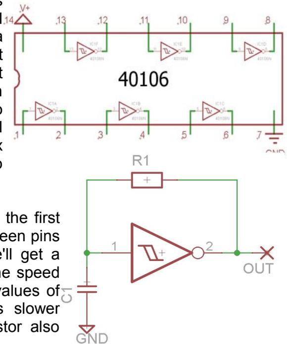
Let's look at the basic *Osc* setup, focusing just on the first gate between pins 1 & 2. If we hook a resistor between pins 1 & 2 and then a cap from pin 1 to ground, we'll get a squarewave output from pin 2 – simple as that! The speed or frequency of the squarewave depends on the values of the two components – a bigger capacitor gives slower speeds (and vice versa), and a large value resistor also gives slower speeds.
