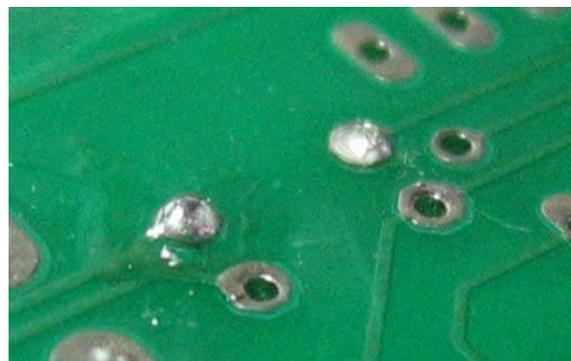
Do the same for the other diode – hopefully you'll be getting a feel for how the solder and iron work and feel... From there we move to the resistors – you may prefer at this point to start placing several components at a time before soldering them all. Though – don't put them all in at once or you'll find all the legs get in the way!
