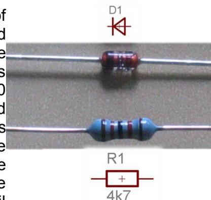
In the bag there are also two **Diodes** – these allow current to flow in one direction only. Note the black ring around one end as this shows which way around to use them. These particular diodes are 1N4148 silicon diodes – the most commonly used in our sort of circuitry.
