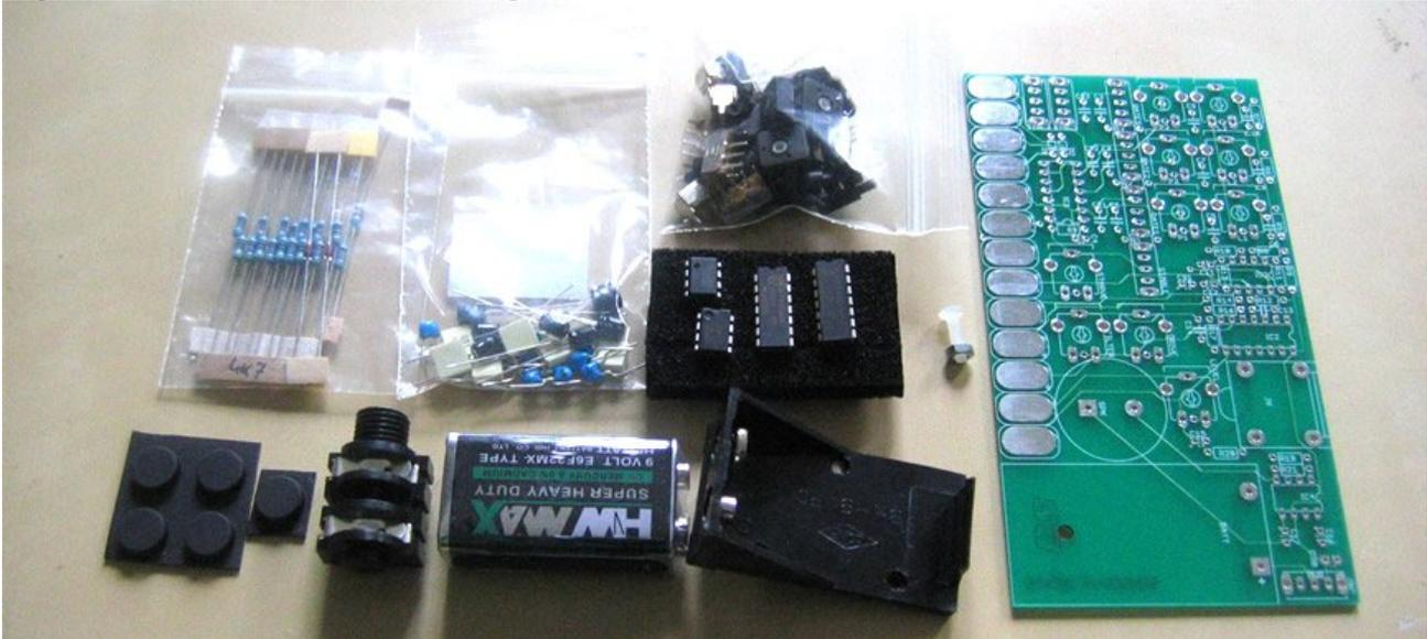
Contents (from top left): Resistors, Capacitors, Dials/Switches, ICs + Holders, Bolt, PCB, Rubber Feet, Jack Socket, Battery + Holder
