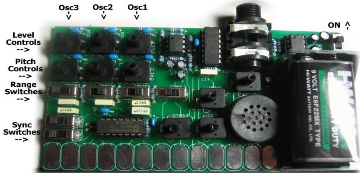
What we've got is: 3 Oscillators -> Mixer -> Comparator -> Distortion -> Output / Amp
