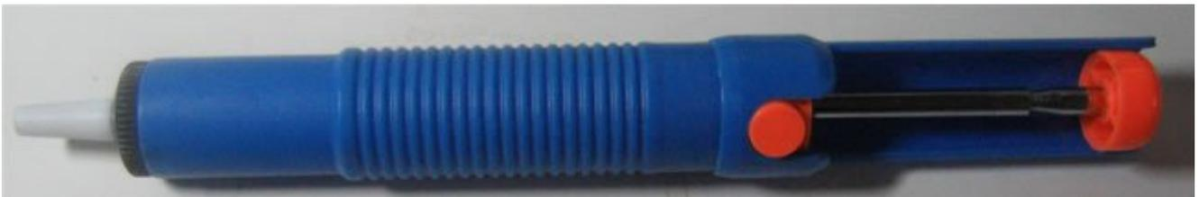
A solder-sucker is vacuum pump which sucks up molten solder. You depress the plunger, use the iron to melt the solder to be removed, place the tip of the sucker by the melted joint and then press the button to suck. Unfortunately, this technique tends not to work so well on fabricated PCBs due to the through-hole plating.
