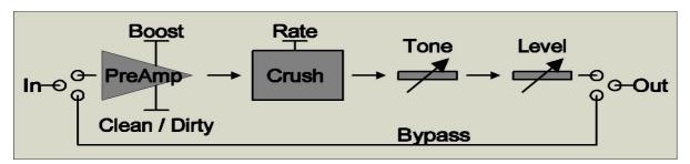
BabyBugCrusher = compact sample-rate reducer pedal.
