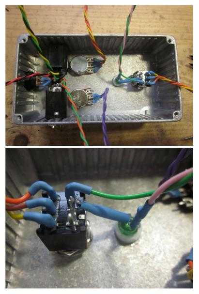
Now the wiring to the PCB.. As mentioned, we made the wires quite long so we could trim them to suitable length later. What I did was position the PCB next to the up-turned box to work out the best length. Trim the wires, then strip the insulation from the end (5-10mm).
