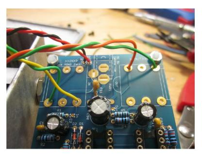
footprints are for TRS sockets with switching contacts, so just ignore the Ring connection and the switching-side connections. [there are also smaller In/Out header points if you prefer]
