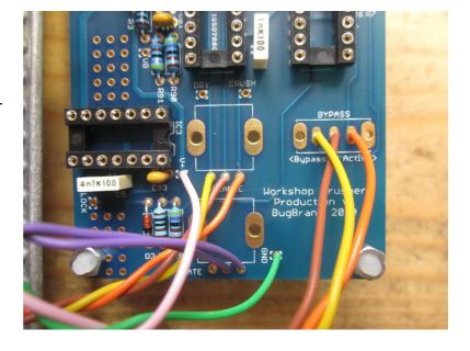
Job done! Put in the ICs (as always, observing static discharge handling as detailed in the main Build Doc). Give it all a test before fitting the PCB on to the base plate with the M3 bolts, nuts and stand-offs, before putting the box together. Plop the knobs on and then HAVE FUN!
