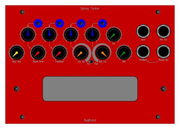
The *BugBrand Spring Tanker* takes a compact Spring Reverb Tank, builds around it the particular drive & recovery circuitry required by such electro-mechanical devices, then surrounds this core with Voltage Controlled analogue processing – the result is a highly playable effects box which massages and transforms the feel of any audio it is fed.
