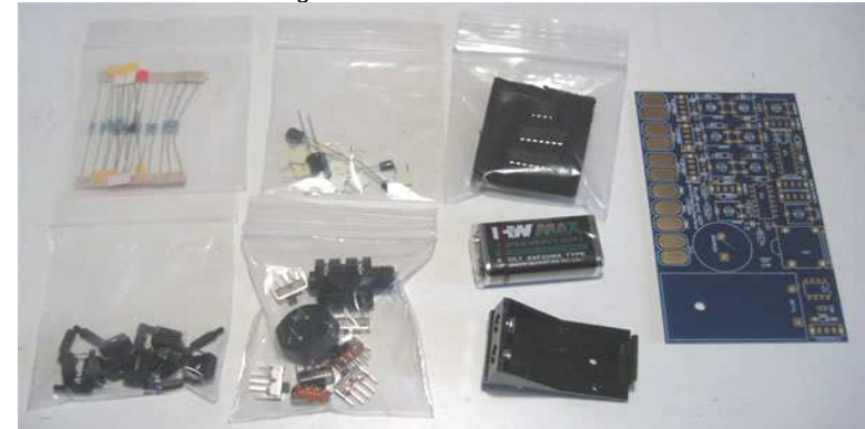
Contents (from top left): Resistors, Capacitors, ICs + Holders, PCB, Dials, Switches + Speaker, Battery + Holder
